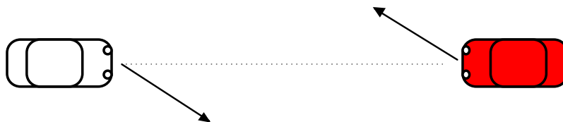
Figure 2. See-and-avoid for collision avoidance in automobile traffic. Each driver looks for conflicting traffic and diverts to their right (or left, depending on the country) as necessary to avoid a collision.
