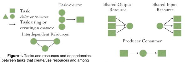
Figure 2. Dependencies between tasks based on shared use of resources.
